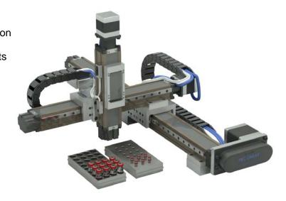
Using three high performance MTB actuators assembled into an XYZ gantry, the new sample transfer system supported a wide working envelope. PBC Linear MT series actuators are driven by steel reinforced timing belt, which ensures high acceleration and fast travel. MT series are composed of an
