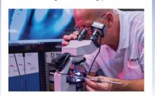
Threadform inspections validate major and minor profile diameters, pitch, flank angle, etc
