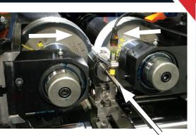
To ensure the highest level of lead accuracy, key process variables such as speed, skew, temperature, and coolant flow, are precisely monitored.
