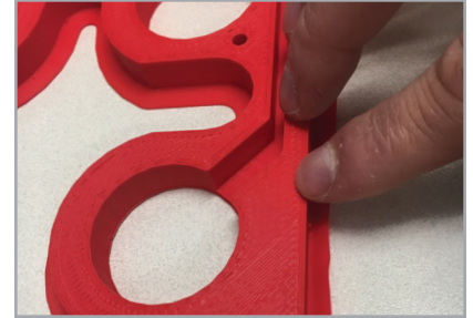
Fixed Print: Solid top layers. Outer walls adhere tightly to the solid layers.
