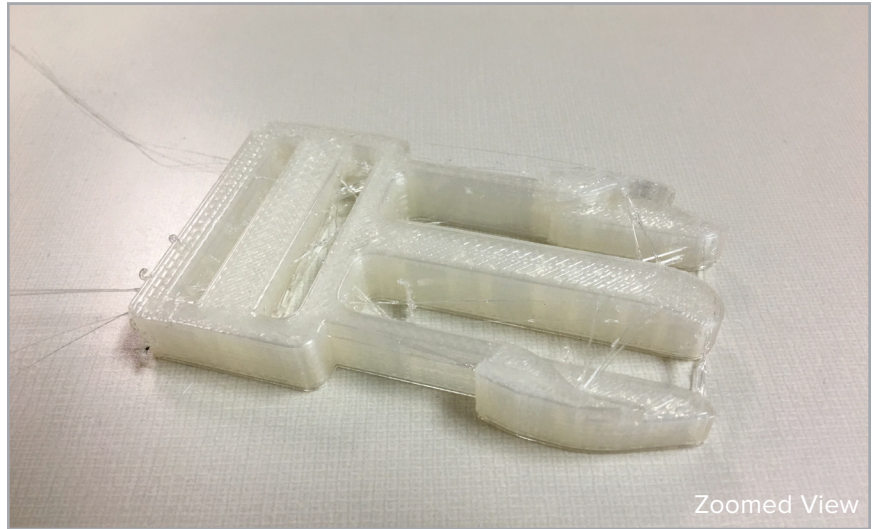
Failed Print: The nozzle leaks and strings between prints.
