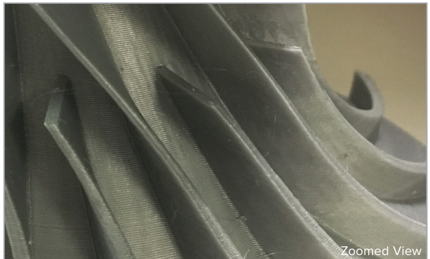
Fixed Print: Smooth layers are essential to a successful print.
